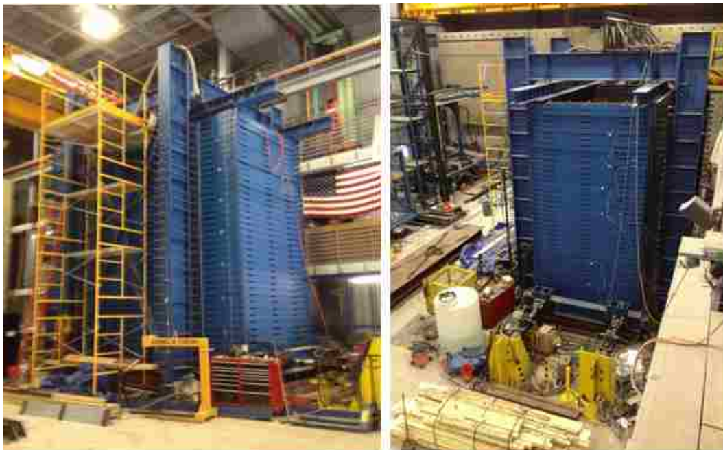
Figure 2-16 Laminar Shear Box and Hydraulic Actuators at the Base (Oakes, 2015)
